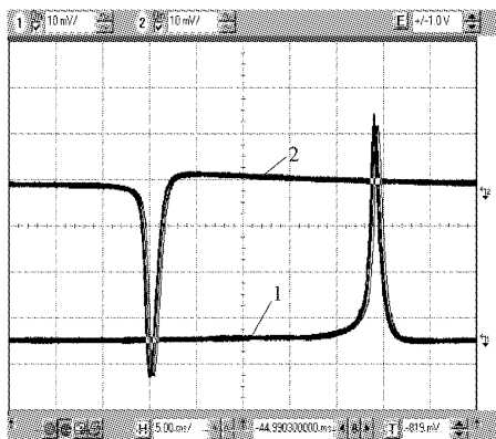
图 7 自由运转, 曲线 1 为扫描 F-P2 腔红外光透射峰曲线, 曲线 2 为扫描 F-P1 腔绿光透射峰曲线(1 min) Fig. 7 Curve 1, fundamental wave transmission through the scanning F-P2 cavity with frequency-stabilized system off (1 min); curve 2: second-harmonic wave transmission through the scanning F-P1 cavity with frequency-stabilized system off (1 min)
